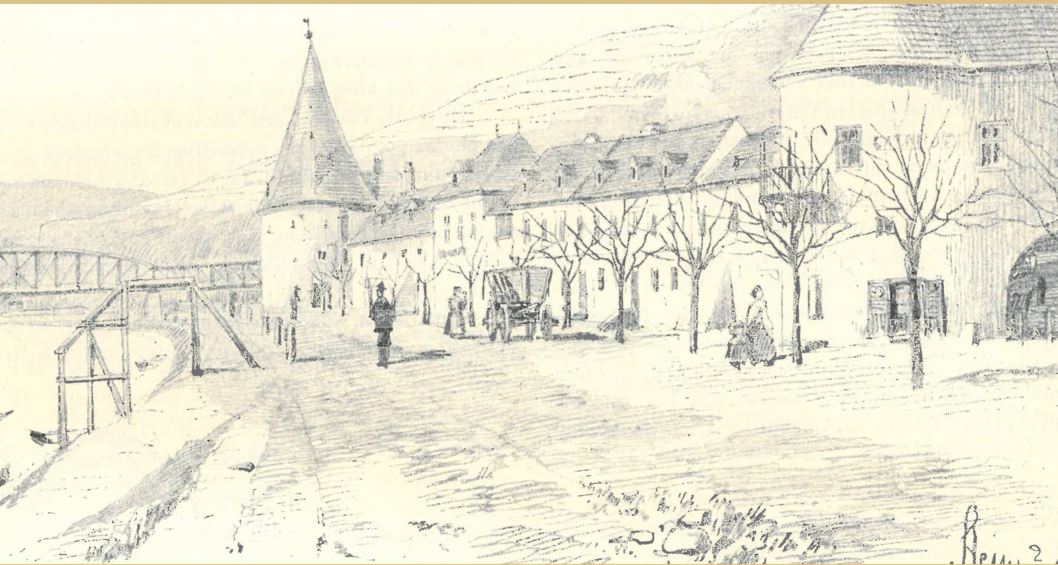
Wachau railway was planned as an embankment track. The drawing makes the impact on the riverine landscape visible which led to a new alignment close to the hills through tunnels.
